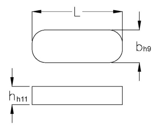
b = 5 h = 5 L = 16.0 Tolerance b = 0.030 Tolerance h = 0.075 Tolerance L = -0.2
